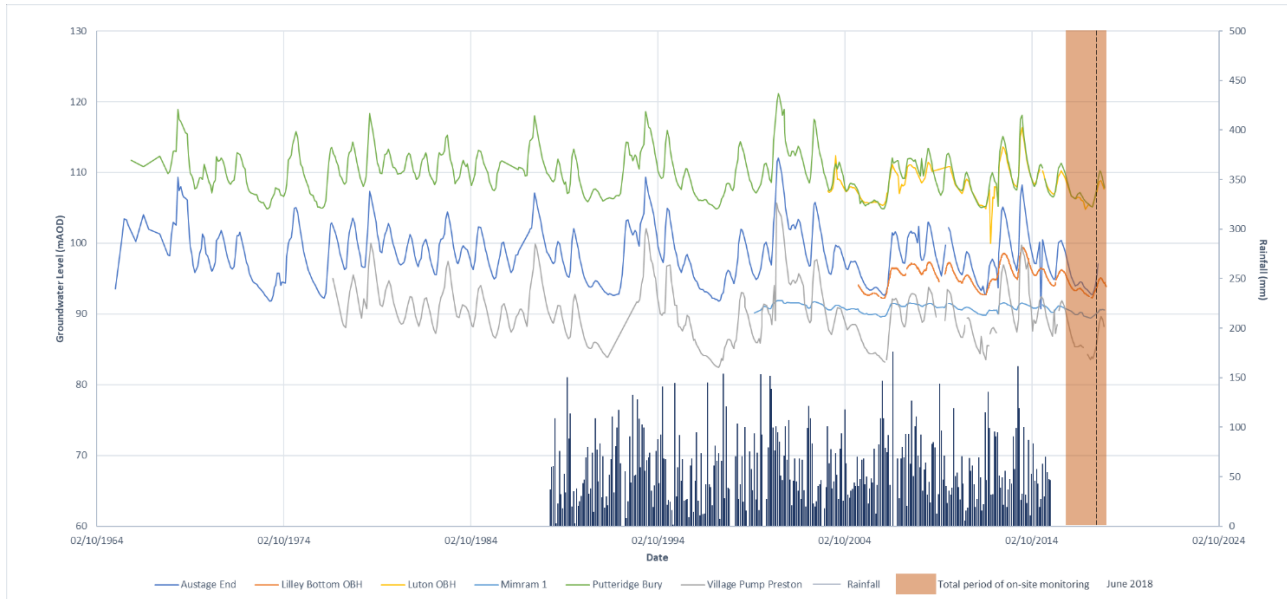
Figure 1: Groundwater elevations in EA boreholes close to the Luton Airport site
